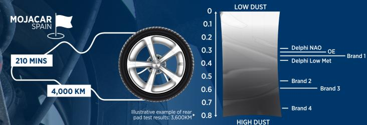
The vehicles, driven in a convoy, took on a 200km circuit that combined the challenges of mountainous and urban driving, each loop taking 210 minutes to complete. Over ten days, each car completed two circuits daily, ensuring a thorough and exhaustive test of the brake pads' dust emissions.
