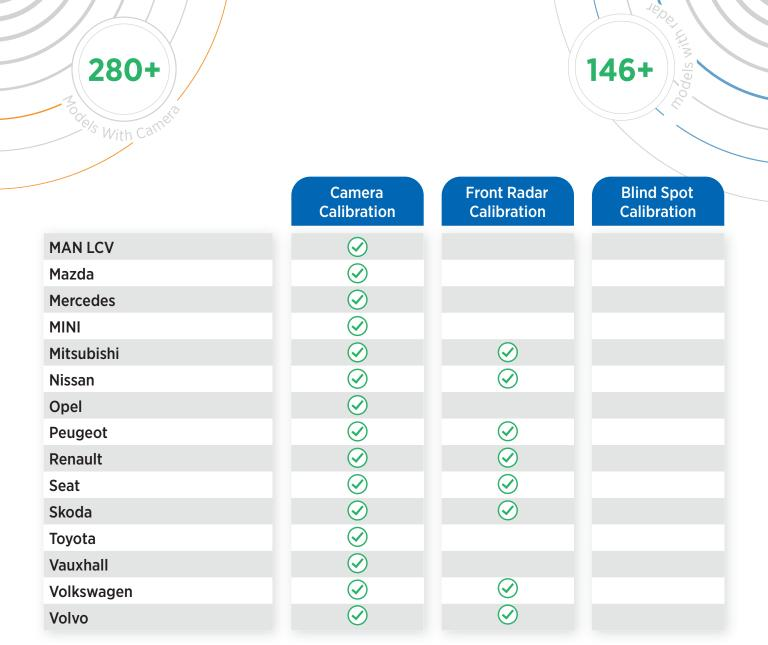
Camera Calibration includes front, rear, 360° overview, and night vision cameras. Our continuous improvement program means our coverage will expand with subsequent software developments.
