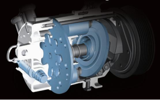
Air conditioning has come a long way in recent years. Not long ago it was a luxury option. Now it is fitted as standard on most new vehicles. The technology has also changed. From fixed swash plate compressors to the latest generation variable displacement compressor technology, air conditioning now requires specialist training and equipment.
